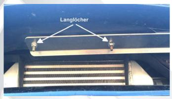
The new bracket has elongated holes so you can perfectly align the bracket / plinth to your front bumper. Please make sure to leave a small (even) gap between bracket and front bumper to avoid damaging the paintwork on your MX-5.
